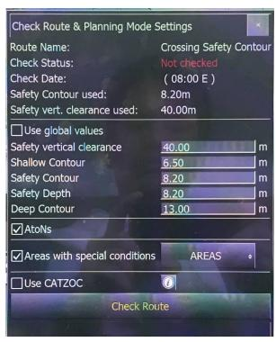
Select Safety Contour in ECDIS and select viewing groups for soundings, seabed features and contours to be displayed. Ensure all obstructions and potential hazards are displayed (safest is to use Display = "ALL")
