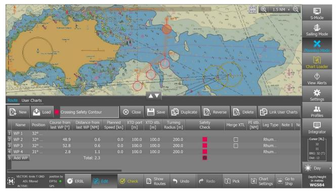
Manually draw (mark-up) Limiting Danger Lines with the User Chart tool using a line demarcating the safe and unsafe areas and marking the latter as Dangerous. Select the User Chart danger alarm in the Chart Alert window for the manually drawn Limiting Danger Lines (and save) so that any approach to this area alarm is activated.
